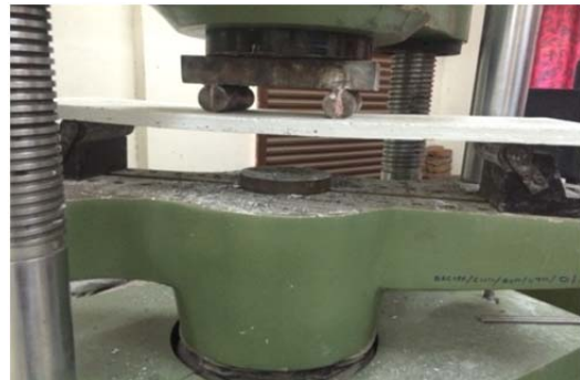
Fig. 8: Two Point Loading System
