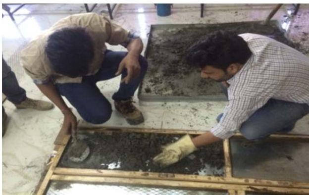
Fig. 6. Mortar Placing (1 st layer)
