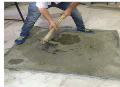
Fig. 3. Mixing of Mortar
