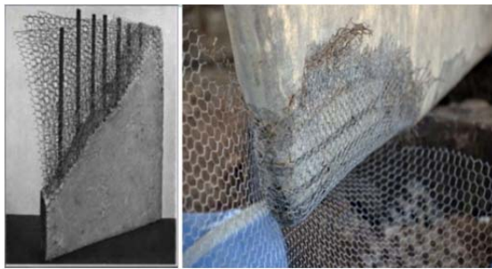
Fig. 1: A usual cross-section of ferrocement panel
